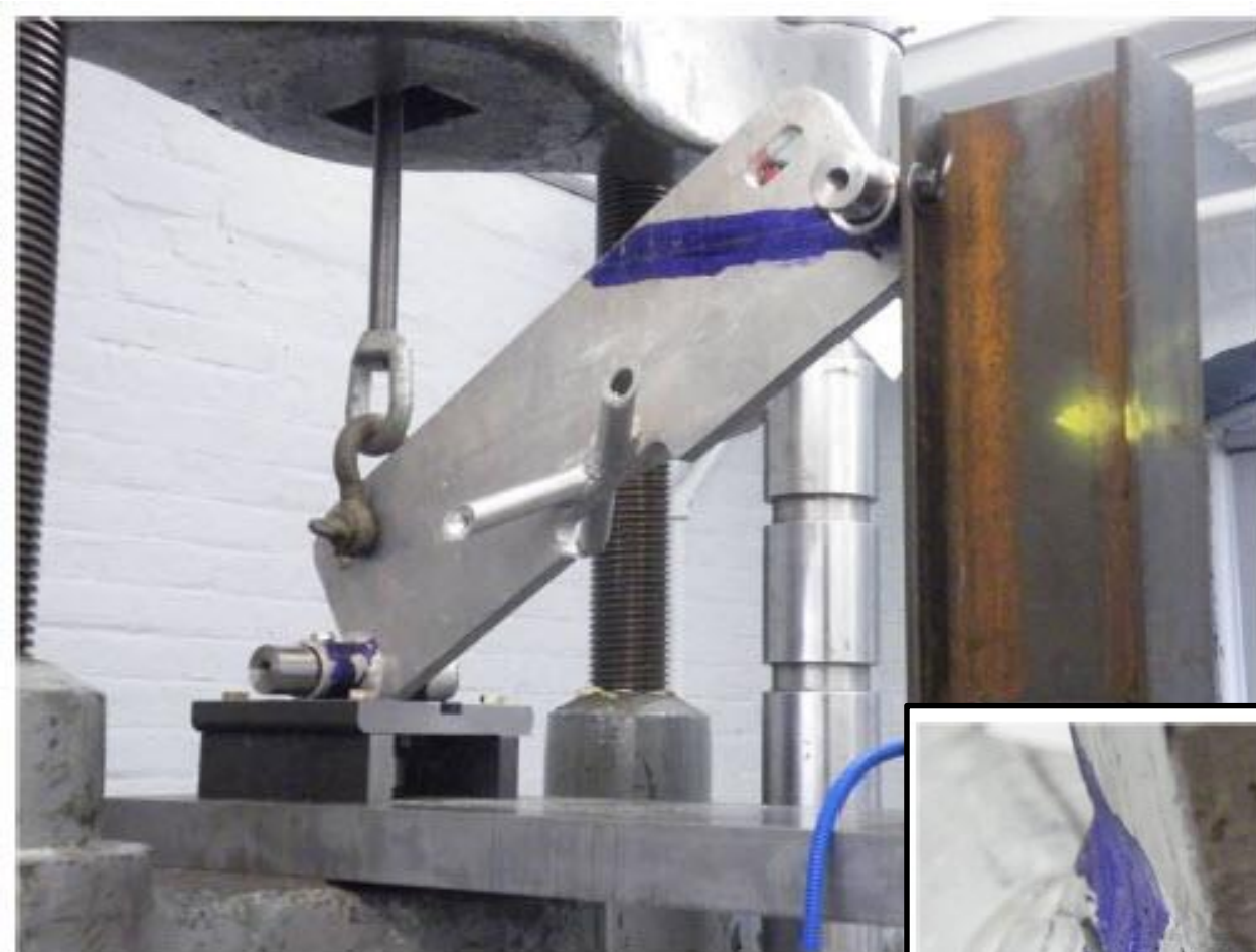
Fig. 6 Fin plate mechanical test setup
